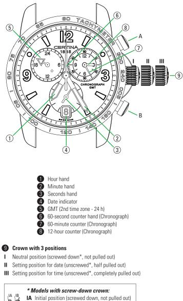
**IB** Neutral position (unscrewed, not pulled out)
